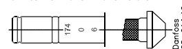
Orifice assembly and filter for flare x flare version for T2 and TE2
